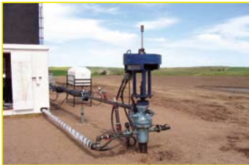
Heavy Oil Well with a Progressive Cavity Pumping System – This rotary system is used for the majority of Rock's heavy oil wells.
